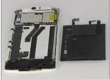
• Use the blue opening tool to carefully pry the battery from the sticky tape that attaches it to the device.
