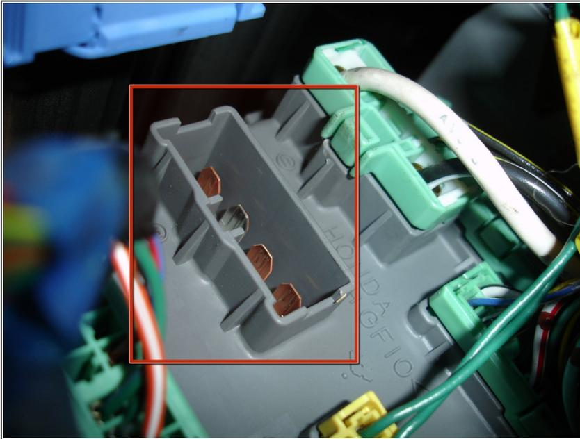
ⓘ At this point you can test the new switch for continuity, just to make sure it's 100% functional before putting it into the car. Follow the same steps outlined in step #7 except use the flat blade screwdriver to switch between ignition positions. You'll notice that the switch clicks just like it does when you insert your key into the steering column ignition. If the continuity tests pass, you can proceed with installing it into your car.
