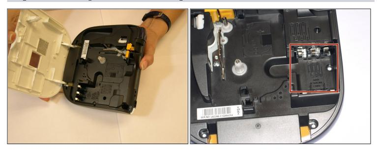
Remove the AAA batteries before you proceed on to replacing the tape cassette.
