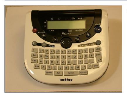
To test the new cassette, make a new label. Press "Shift" and "Print" to feed the tape, then use the cutting lever on the upper-right corner of the machine.
