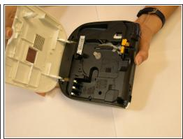
• First, flip over your label maker and push down on the top part(by the face plate) and push on the circle part with ridges. Next open the label maker carefully to prevent any damage.
