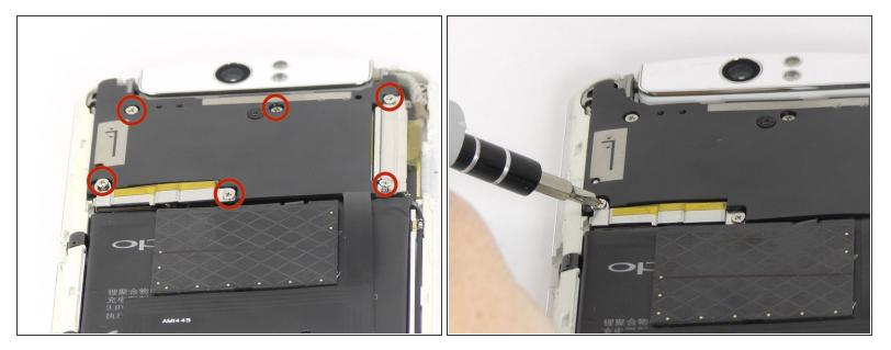
Remove the six 4mm long screws holding the motherboard in with the ph0 Phillips head screw driver.
