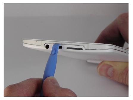
Insert the plastic opening tool into the crevice. The back cover is most easily opened by starting at this location.
