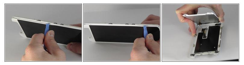
Insert the blue opening tool into the crevice between the screen and the main body of the phone.
