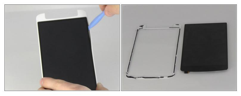
Insert the blue opening tool in between the black screen and the white border and slide it around the edge of the black screen.
