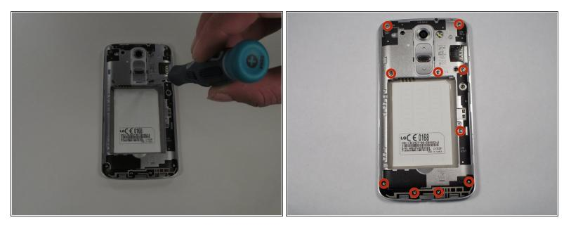
Locate 10 screws and remove each one using a screw driver.
