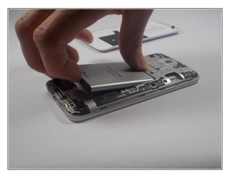
• Remove the battery from the battery bay by prying with your finger at the groove on the lower end of the battery bay.
