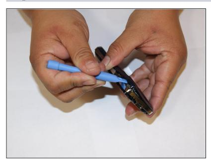
Remove front casing by sliding a plastic opening tool between the chrome layer and the top cover.
