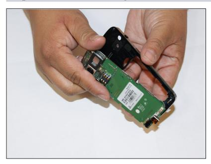
Remove the back casing by taking the motherboard and back casing and pulling them apart.
