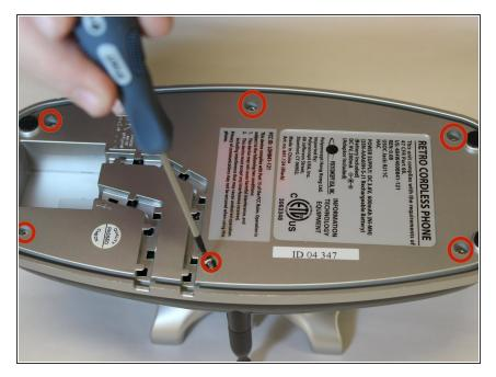
Using a Phillips #00 screwdriver, remove the six 7mm screws from the base plate.
