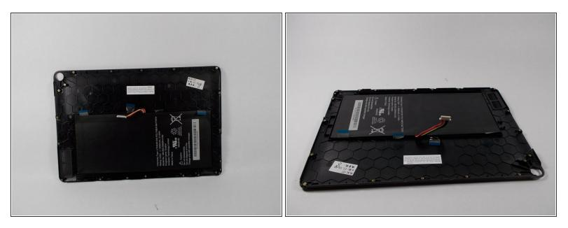
• Pry battery off of bottom frame using plastic opening tool.
