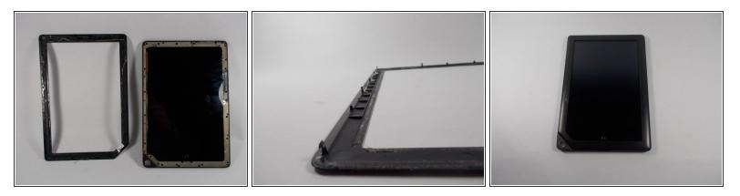
Wedge the plastic opening piece underneath the bottom left hand corner of the front frame. Pry the frame off of the Nook.
