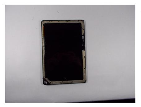
• Carefully remove center chassis from bottom frame.
