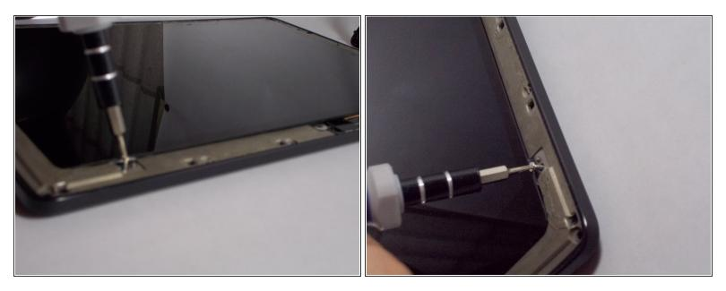
Remove every visible screw tying the chassis to the bottom frame using the T-4 attachment for the screwdriver in the iFixit screwdriver kit.
