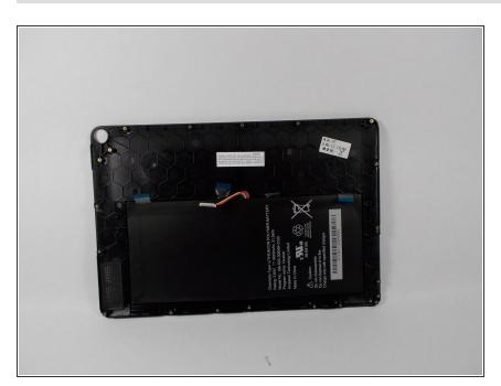
Apply glue to the bottom side of new battery. Re-insert new battery onto bottom frame and allow to dry.
