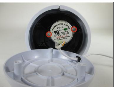
Remove the two 10mm screws using the Phillips #0 Screwdriver.
