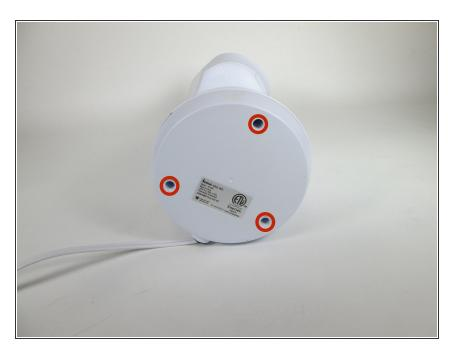
Remove the three 12mm screws using the Phillips #0 Screwdriver.
