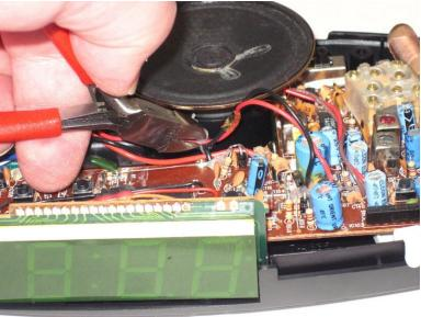
Using the wire cutters, carefully cut the plastic wire tie.
