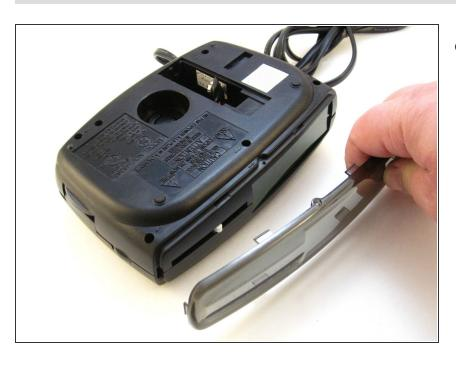
Gently pull the liquid crystal display (LCD) cover off.
