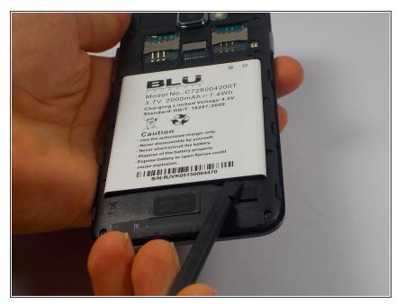
• With the back panel off, you should see a large white rectangle. This is the battery. Slide the spudger under the indent on the bottom right of the battery and pull it up.
