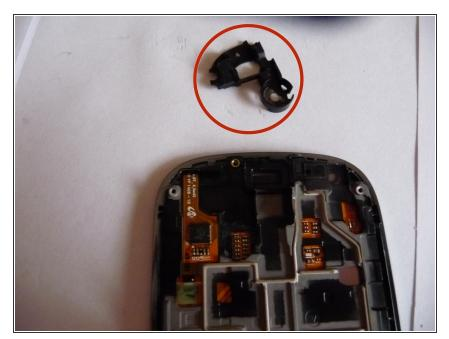
Using a plastic opening tool, remove the support piece.
