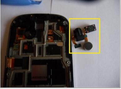
Using a plastic opening tool, carefully remove the headphone jack (red)/earpiece (red)/vibrator (orange) assembly. This is removed as a single unit. Be particularly careful with the thin ribbon cables connecting them together as they can be easily torn.
