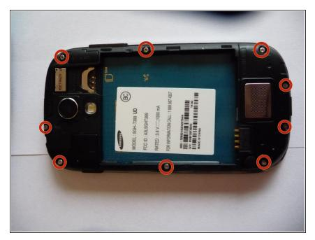
Using a Phillips #0 screwdriver, remove all nine (9) screws attaching the midframe to the front of the device.
