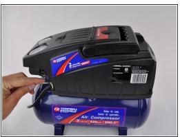
Unscrew the four 1cm long shroud screws using a 6mm Allen Wrench.
