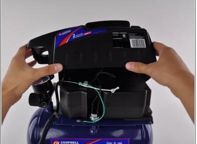
Remove the plastic shroud from the compressor.
