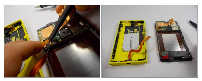
• Once the metal clip is removed, gently pry up on the ribbon cable connection, located underneath the metal clip you have just removed.
