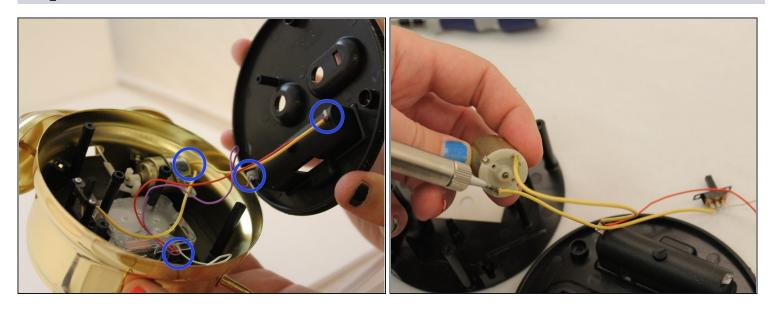
Use a soldering iron to melt the solder on each wire connection to safely remove the wires.
