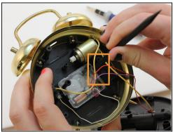
• Use a spudger to open and detach the wiring box from the clock. Insert the flat end of the spudger on both sides of the box, gently pry it open and detach it from the clock. Be careful while handling the box and clock to avoid any damage or injury.
