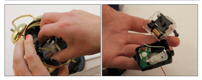
• To replace the wiring box, use your hand to remove the old one and install a new one in its place.
