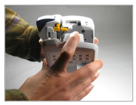
Remove the back cover of the device by simultaneously pressing down on the indication arrows on the top center, then pulling toward you.
