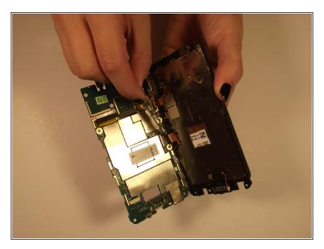
Disconnect the two aluminum flex cables
