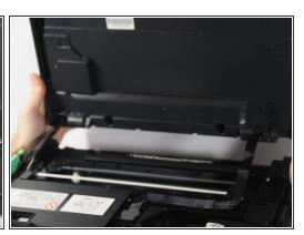
To remove scanner head, open it halfway as possible and slide the hinges out of place and the head will be removed.
