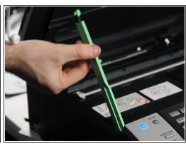
Twist green section to allow the scanner head to have a full range of motion.
