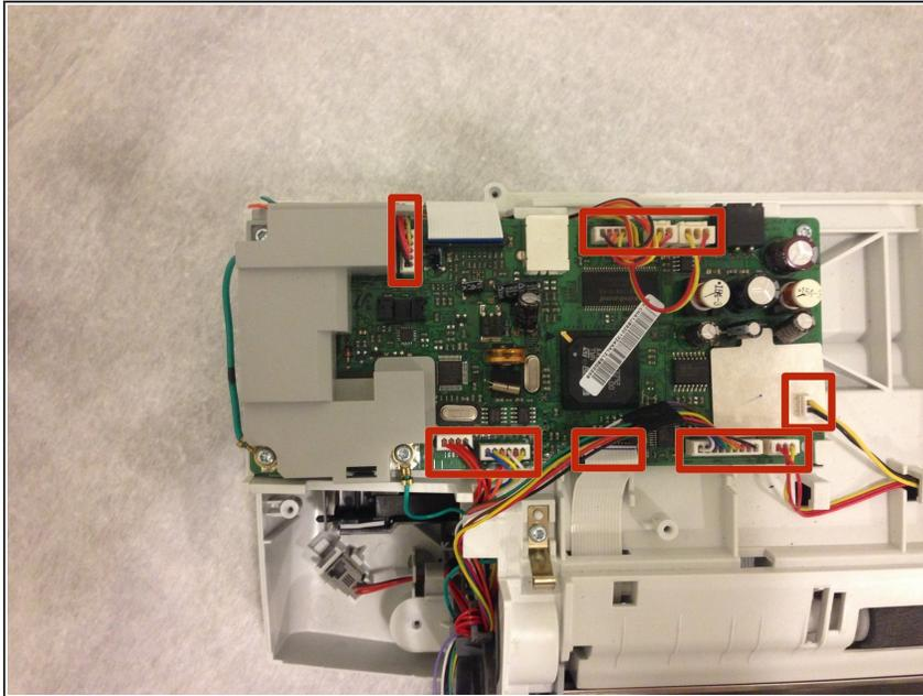
**⚠** Carefully unplug all of the plugs that are connected to the main motherboard indicating in the picture.
