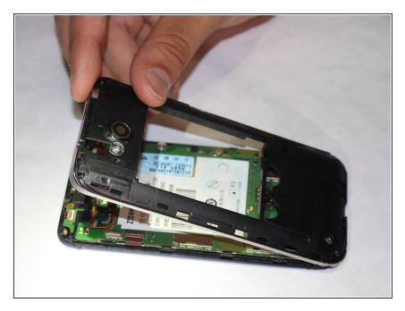
Separate the back panel from the motherboard.
