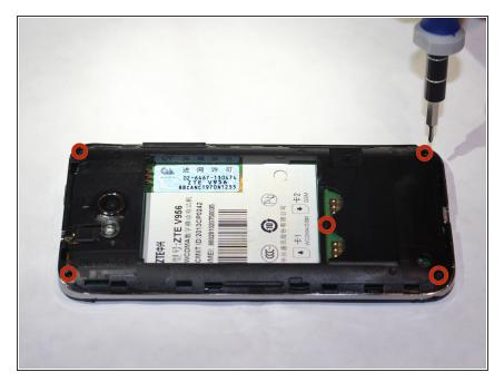
Remove the five 4mm Phillip's #00 screws, circled in red, from the back panel.
