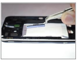
Using a pair of tweezers, remove the volume button by unlatching the two white bands holding it in place.
