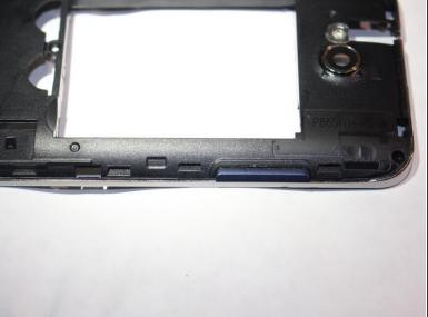
• Either replace the volume button with a new one, or reinsert the old one using a pair of tweezers. It should look like the pictures when inserted properly.
