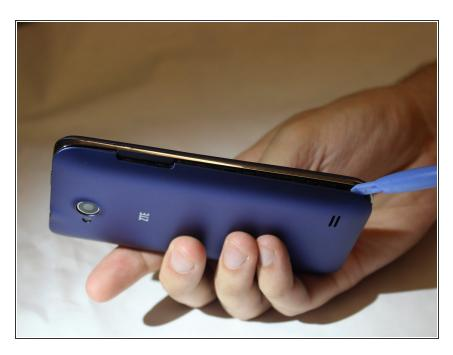
Using your finger nails or a spudger, remove the back panel from the phone.
