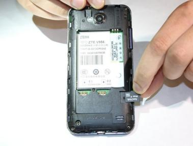
• Using your fingernails or a spudger, remove the phones battery and microSD card.
