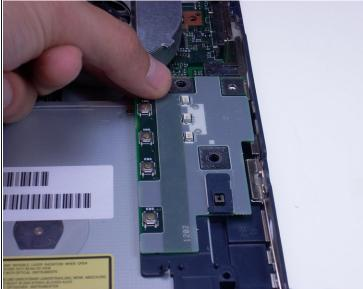
As shown by the photo, remove the small green computer part by pinching the top with your fingers and gently lift it away from the laptop.
