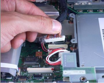
Setting screen next to the base of the laptop, pinch the connecting cable with your fingers and gently pull connecting cable from monitor.
