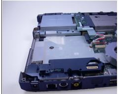
Using your fingers, slowly slide the optical drive out of the laptop, towards you, until you are able to completely lift it away from the computer.
