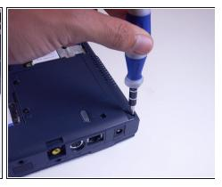
Using a Phillips screwdriver, unscrew and remove 5 B20 screws, located along the corners of the bottom of the laptop.
