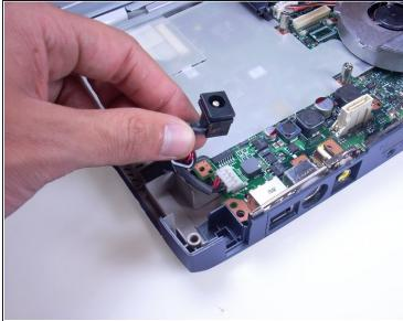
• Lift DC adaptor by sliding upwards out of the laptop and hold out of way.
