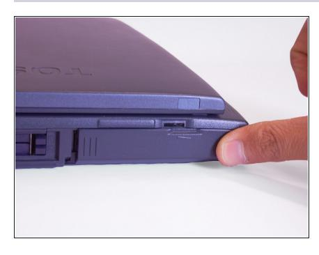
Placing your finger on the raised grip, push the battery casing to the right. It will slide over.
