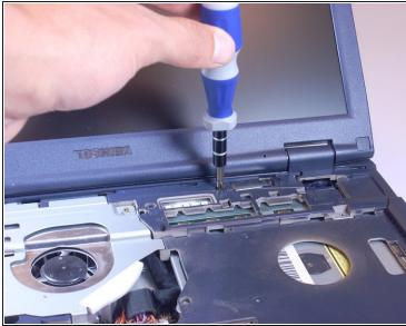
• Using a Phillips screwdriver, unscrew and remove two screws labeled B25 located closest to the screen.
