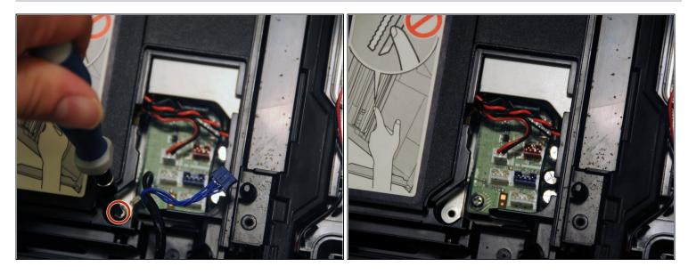
• Unscrew the 12.1mm screw to remove the ground wire.
