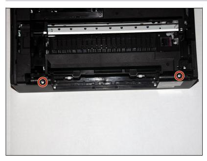
• Unscrew the two 14.1mm screws holding the rear panel in place.
