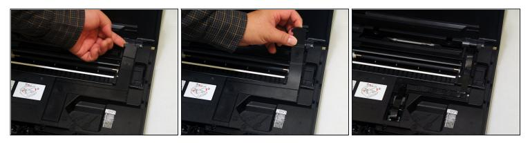
• Use the exposed portion of the panel to begin to lift the panel away from the back of the device.
