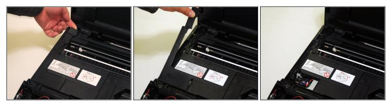
• From the back of the device, use the exposed portion of the panel and gently begin to remove the panel away from the device.
