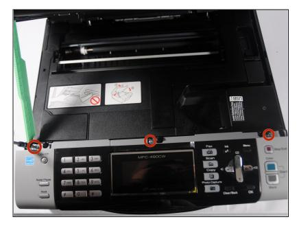
Use a Phillips #2 screwdriver to remove the three 12.1 mm screws holding the control panel in place.
