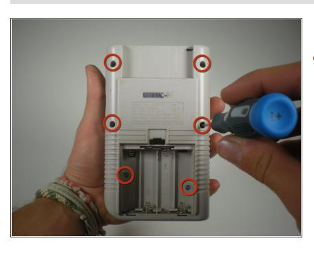
Remove the six Triwing screws from the back of the device.
