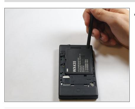
Gently pry out the battery using the spudger
