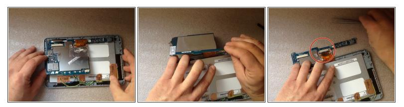
Lift the board from the side of the battery connector and turn it around the display connector on 360 degrees.
