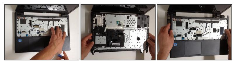
• Carefully separate the upper cover and remove it.
