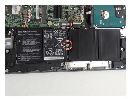
Remove the single Phillips 0 screw securing the battery.
