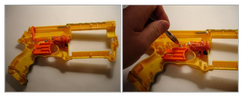
• The trigger is held in place by a sole Phillips screw. It also has a small spring for that authentic handgun "springy" feeling...
