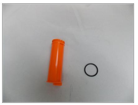
Use a pair of tweezers to remove the O-Ring from the top of the air plunger.
