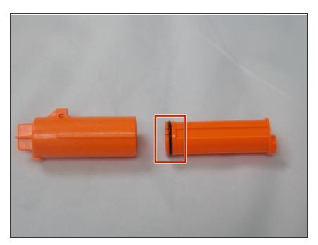
Once you have the air plunger removed, locate the O-Ring by pulling the two pieces of the air plunger apart.
