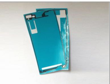
Before installing the new cover, you must clean the phone from the old adhesive tape and install a
