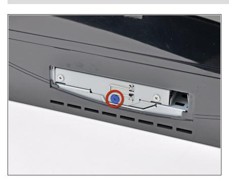
Remove the blue 8 mm Phillips screw securing the hard drive cage to the chassis.
