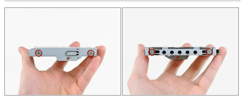
• Remove the four 4.3 mm Phillips screws securing the hard drive cage to the hard drive.
