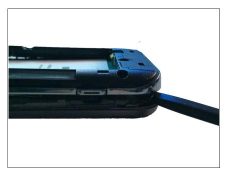
Using a spudger or plastic pry tool, slowly go around the phone between the display & rear housing to release the clips.
