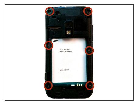
Remove the 6 Phillips head screws that hold the rear housing in place.
