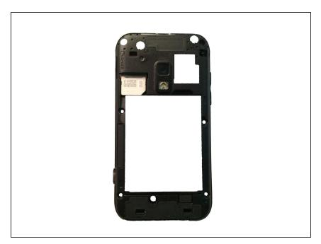
Lift the rear housing from the display assembly.
