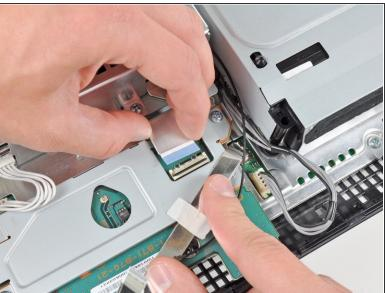
Use your fingernail to flip up the retaining flap on the Wi-Fi/Bluetooth ribbon cable socket.
