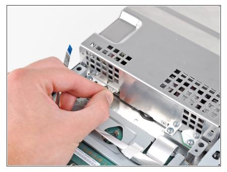
Pull the DC-In cables toward the front of the PS3 to disconnect them from the power supply.
