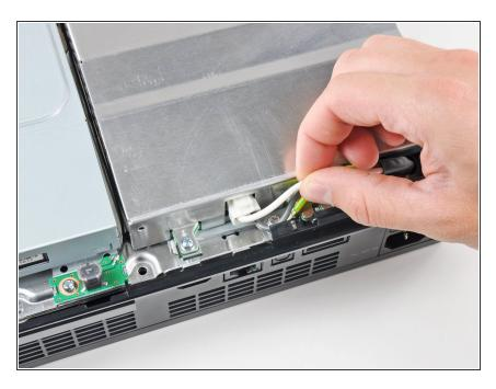
Lift the AC-In cables slightly away from the rear cover for clearance to access the AC-In connector.
