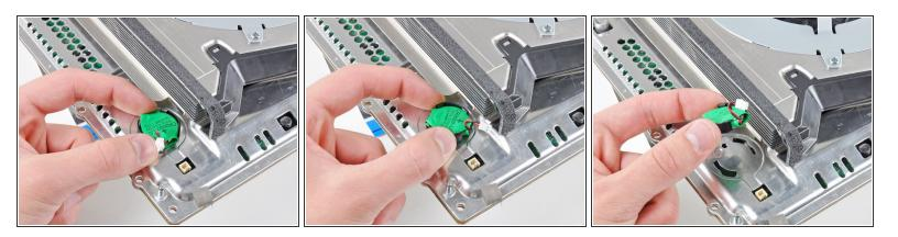
Rotate the PRAM battery counter-clockwise and remove it from the chassis.
