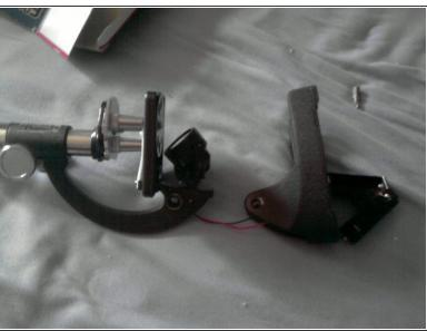
Now, remove the big Phillips screw here (actually, you can loosen it then remove the nut in the other side). Don't be worried if it's a little hard to pull the screw.
