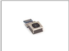
Release rear camera connector and remove it.
