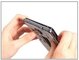
Cut LCD screen sticker, loosen clasps around battery slot and push the whole front assembly out from middle housing.
