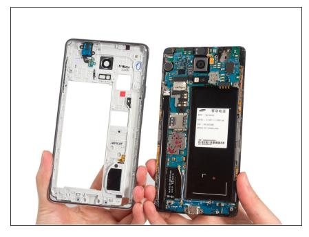
We can see the motherboard now and the rear camera is connected by a connector on the back of motherboard. So we have to remove motherboard before removing rear camera.
