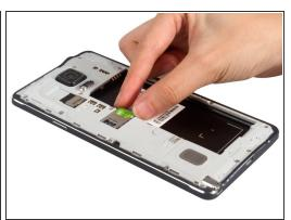
Take away the back cover and battery easily. Don't forget to remove SIM card and S Pen.
