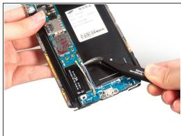
Release connectors which connecting with motherboard.
