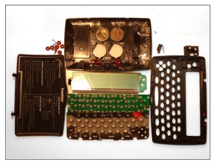
Here is a full view of the disassembled Franklin MWD-460A Electronic Dictionary.
