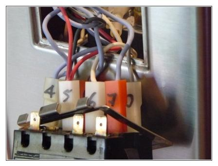
Make sure you label each connector. It's possible to use the wiring diagram if you forget, but much easier if use labels.
