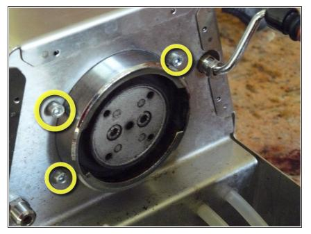
Remove the four bolts holding the boiler assembly into the case of the machine. You'll need the smaller of the allen keys / wrenches for this. (the diagram only shows three of the bolts, the fourth is obscured).
