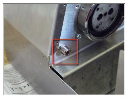
Now we disconnect the tubing that leads to the overflow pipe. Locate the external overflow pipe connector.
