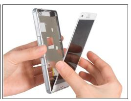
Separate the LCD screen with earpiece from midframe. See the detail on <u>Sony Xperia Z3</u>
