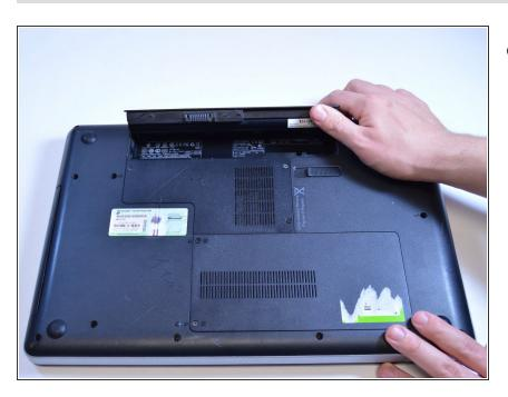
Carefully remove the battery from its compartment.
