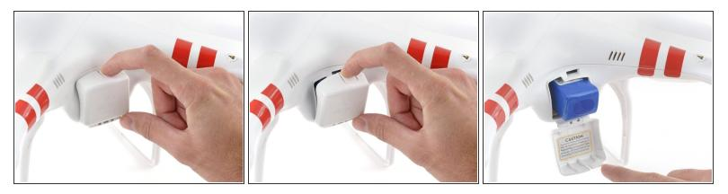
• Press down on battery door release tab to flip the battery door open.
