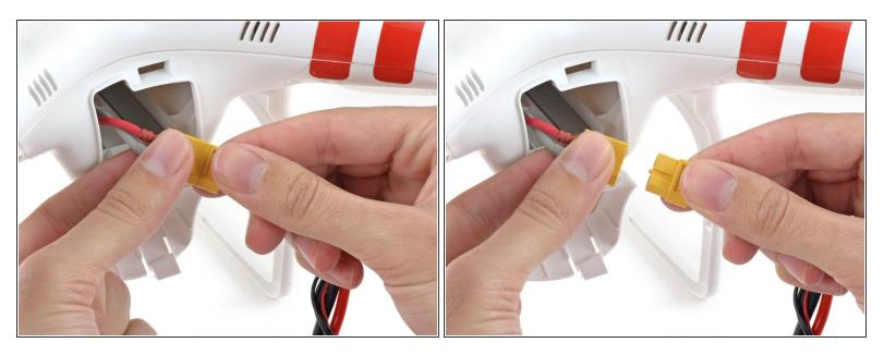
• Pull the two halves of the XT60 power connector apart.
