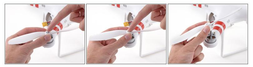
• Gently press down the motor shaft and lift the propeller up to remove it.
