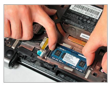
Push both tabs outward to release the memory module
