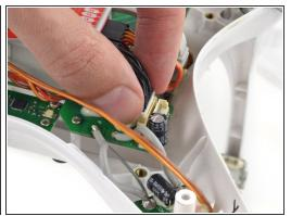
Pull the gimbal wire through the case bottom shell and plug in the connector to the G8 plug on the mainboard.
