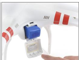
Press down on battery door release tab to flip the battery door open.
