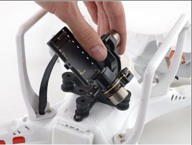
Place the gimbal on the mount with the front facing the same side as the battery cover.
