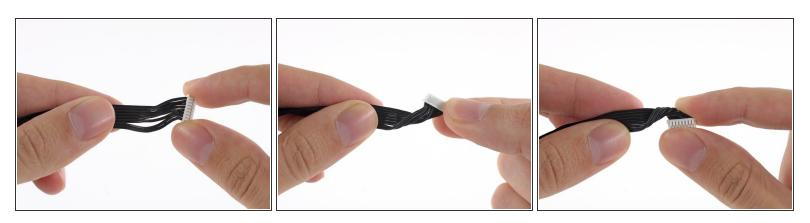
Twist the molex and cable as shown to prepare it for insertion through the case bottom shell.
