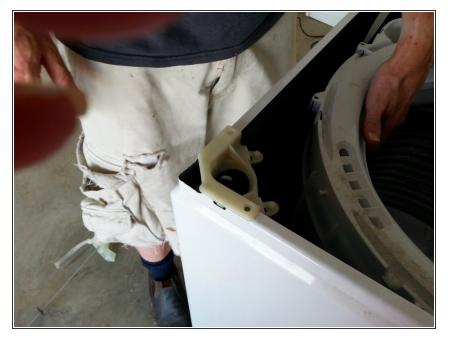
Place your left hand under the drum rim and support it. Remove and replace one rod at a time. You don't want the weight of the drum on the motor and pump below as you may break something underneath. By replacing them one at a time, the other three can help support the weight of the drum.
