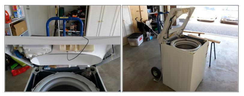
I used an old coat hanger to suspend the plastic cover out of the way by hooking it onto the trolley that I used to move the washing machine. This gives you access to the 4 rubber straps and 4 suspension rods.
