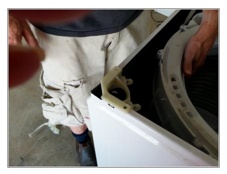
To remove the rods lift the plastic hanger off the chassis and then jiggle the bottom part of the rod out of the slotted holder. There are no fasteners holding the rods in place. Its just the weight of the drum holding them in place.
