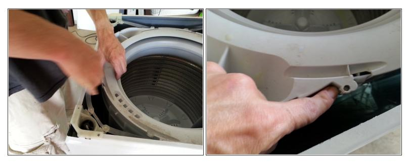
• You will see there are four rubber straps, one in each corner. I decided to replace these as well just to be on the safe side. When the old and new rubber straps were placed next to each other there was a significant difference in length. Just pull them straight off.
