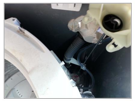
• There is a clip half way down the rear right rod that needs to be undone. You also need to move the hoses and electrical looms out from under the plastic hanger prior to removing the rod. To remove the rods lift the plastic hanger off the chassis and then jiggle the bottom part of the rod out of the slotted holder.
