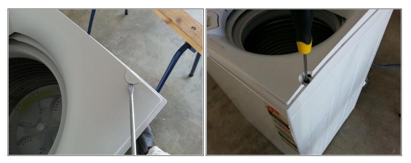
• Simply pry off the plastic screw covers then unscrew the two forward screws. Note there is no need to remove the cover, just tilt it backwards on its hinge to gain access. Be careful with hoses and electrical wires at the back of the cover.
