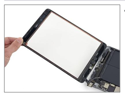
• Lift and remove the front panel from the iPad.
