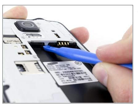
Use a plastic opening tool to loosen the clasps around the battery housing.
