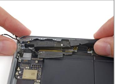
• Push the speaker with the flat end of a spudger to begin sliding it out of its recess in the rear case.
