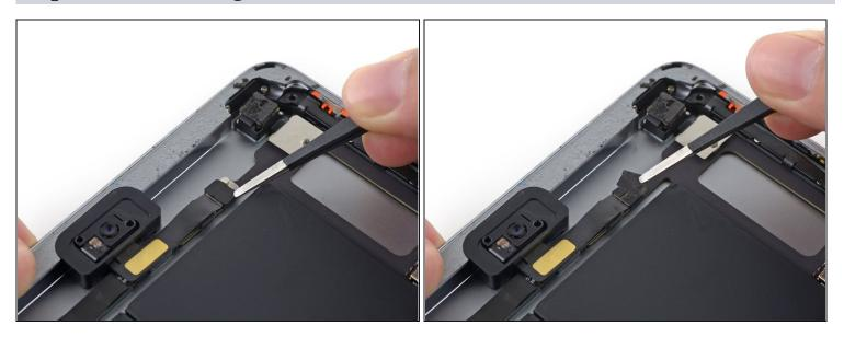
• Use a set of tweezers to remove any tape covering the front-facing camera cable clips.
