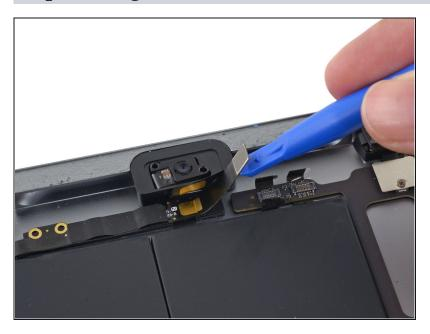
Lift the headphone jack cable up out of the way of the logic board.
