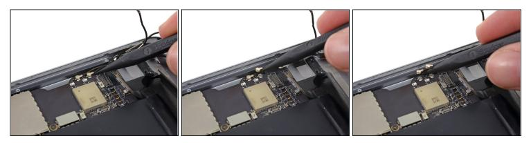
• Use the point of a spudger to lift the two antenna cable connectors straight up off of their sockets on the logic board.
