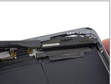
• Push from the Lightning connector end with the flat end of a spudger to free the speaker from the lip of the rear case.
