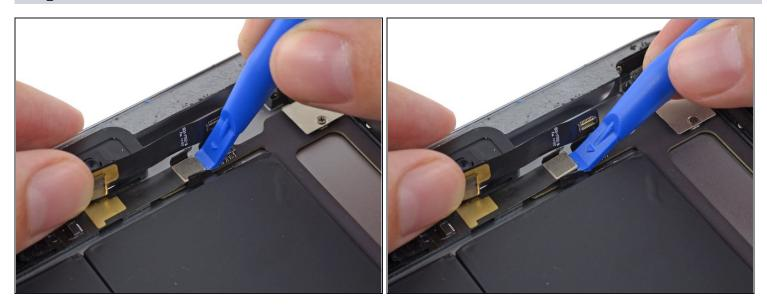
• Use a plastic opening tool to pry the headphone jack cable's connector up from its socket on the logic board.
