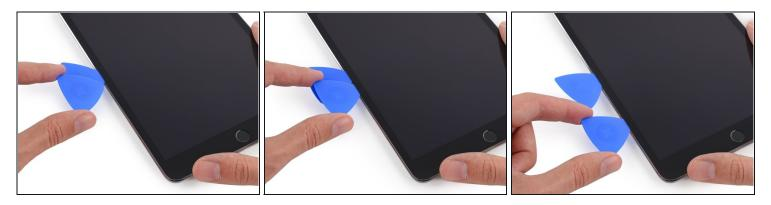
Place a second opening pick alongside the first and slide the pick down along the edge of the iPad, releasing the adhesive as you go.
