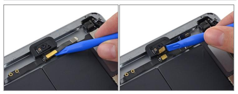
• Use a plastic opening tool to gently fold the front-facing camera cable upwards (roughly at a 90-degree angle), exposing the bottom side of it.
