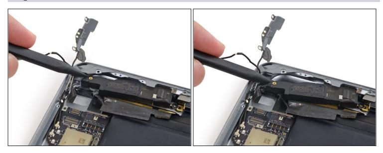
• Insert the tip of a spudger into the gap between the left speaker and the bottom left side of the rear case.
