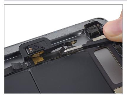
Remove any tape covering the headphone jack cable connector.
