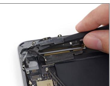
• Use the flat end of a spudger to cut the foam adhesive securing the antenna to the right speaker.
