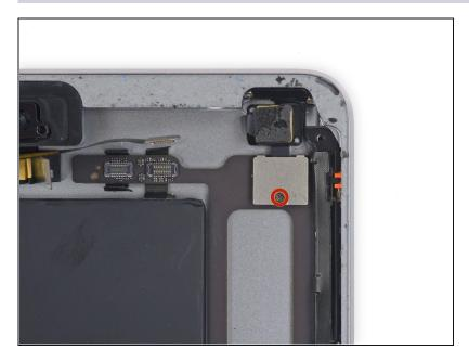
Remove the 1.4 mm Phillips #00 screw securing the rearfacing camera cable bracket.
