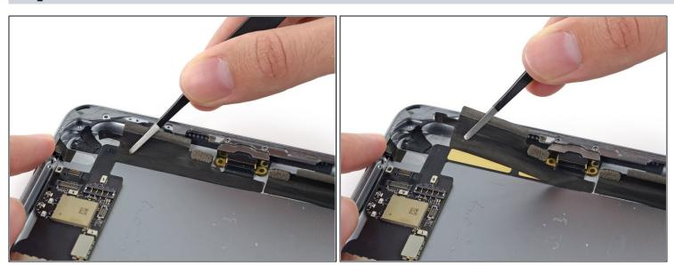
• Peel up the tape covering the Lightning connector cable.
