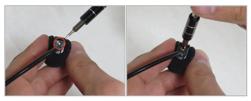
Using a Philips #0 screwdriver, unscrew the 4-mm-long screw that attaches the windscreen to the microphone.
